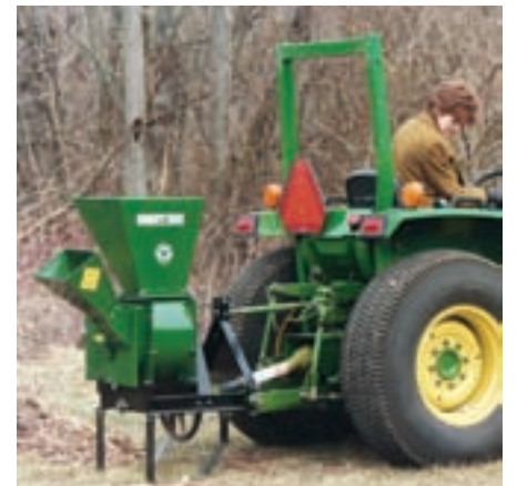
TPH122: Lowered position for operation
